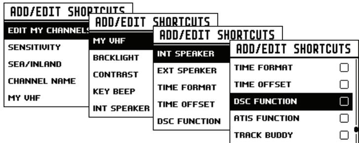
→ **Note:** The MY VHF page is only available to the operator when enabled as a shortcut - it can't be accessed via another menu. Its purpose is solely for displaying radio information in one easy to access location.
