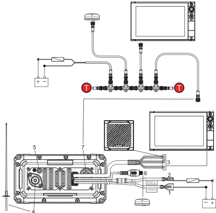
1. Battery - (black): connect to vessel's negative busbar
