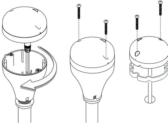
To **pole mount** the external GPS-500 antenna, you will require a 1-inch 14 TPI thread pole:
