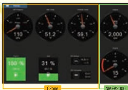
CZone, engine, navigation and various NMEA2000 data can be laid out in the same screen.
